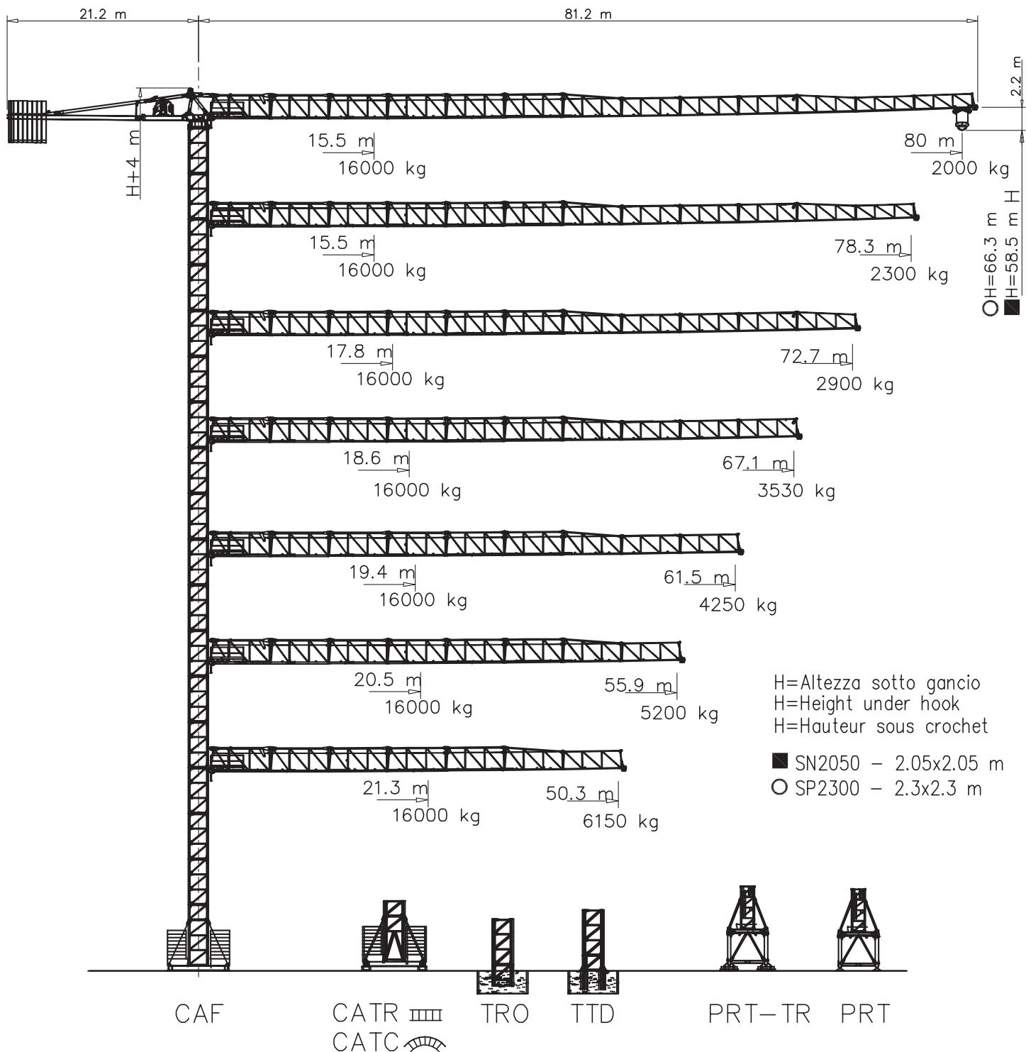
Torre/Reazioni – Masts/Reactions – Mat/Réactions – Maste/Eckdrücke – Mástil/Reacciones – Tramo/Reacções
