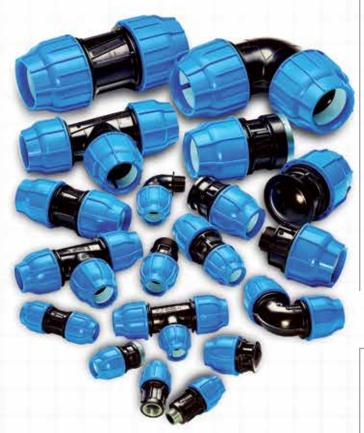
**MAGNUM®** is a system of polypropylene mechanical compression fittings specifically designed to join PE pipes with U-PVC, PVC-C, PP, PE-X, copper, lead and steel pipes through a combination of specific quick release connections and several patented tightening mechanisms.
