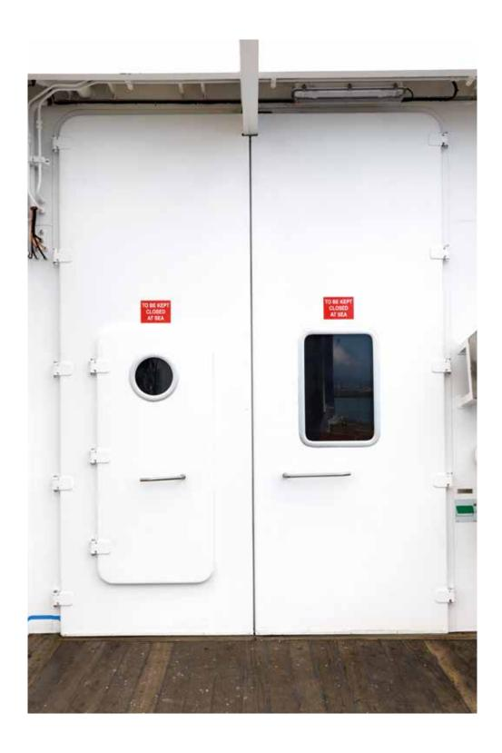
Double-leaf hangar gate with an insulated, aluminium access door that is Spraytight and adapted to the hoist girder.
