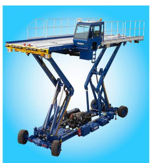
Timsan KL18500 Military Aircraft Loader is capable to load and unload all types of pallets, ULD's, loose and Air-drop cargos and vehicles, to all cargo aircrafts and has the following listed advantages
